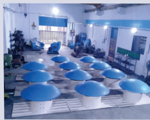
Mechanical Roof Exhaust Fan
